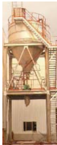
Steam cooled cyclone (above 100 T/H capacity) Power Plant use Automatic ASH BIN pneumatic pump to collect ash to the fluidizing Ash silo for automatic discharge to the truck. (Totally closed system)
