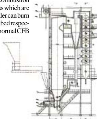
Circulating Fluidized Bed (CFB)
