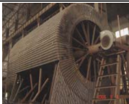
Steam cooled cyclone (above 100 T/H capacity) Power Plant use Automatic ASH BIN pneumatic pump to collect ash to the fluidizing Ash silo for automatic discharge to the truck. (Totally closed system)
