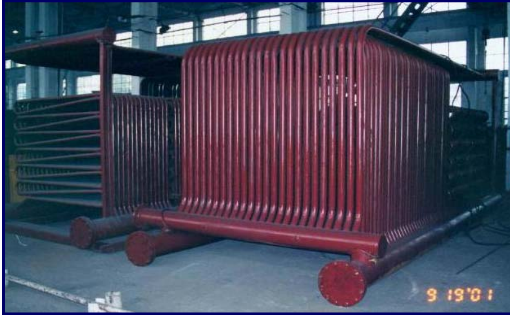
Multi tubular type heat exchanger vessel, designed for coal combustion, which is more efficient than the coil type
