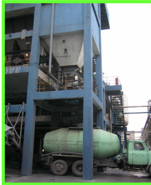
Auto ash discharge to truck
