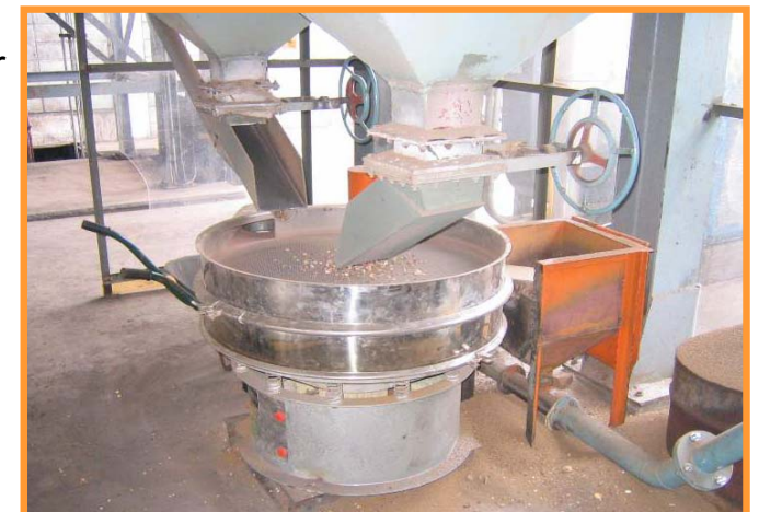
Foreign materials and stones are separated by this screen vibrator
