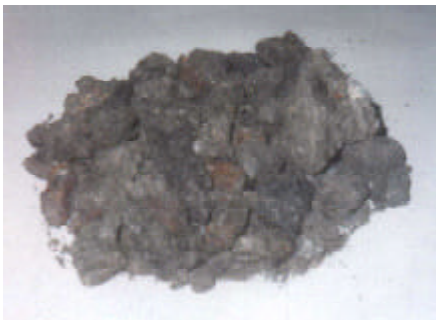
Rough & coarse ash from Chain Grate
